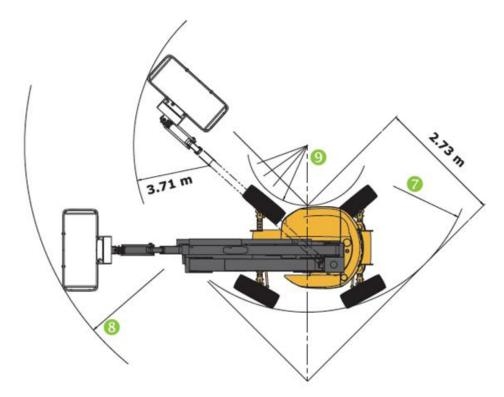
Working height: 16.40m Platform floor height: 14.40m Max. outreach: 8.95m
